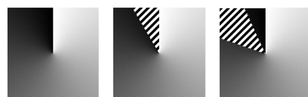
Fig. 3: Two k -flat zones which overlap where k = 16 [2]
